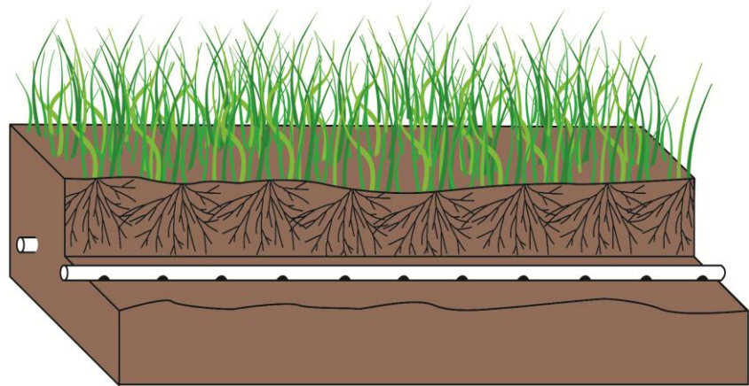
Figure 3. Cross-Section of a Drip Irrigation Effluent Dispersal System
