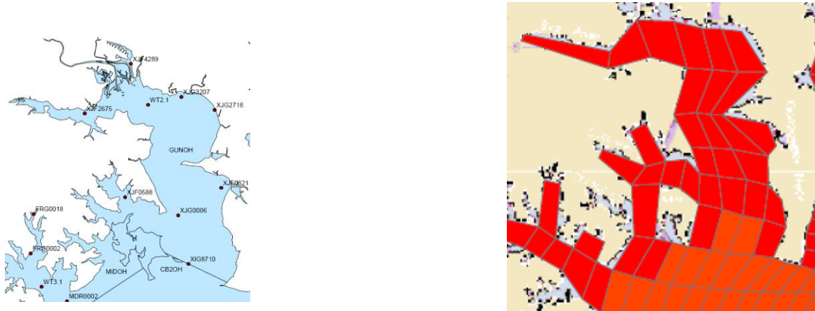
Figure N2-8. The location of the Gunpowder River (a) and the Chesapeake Bay Water Quality Model representation of Gunpowder River (b).
